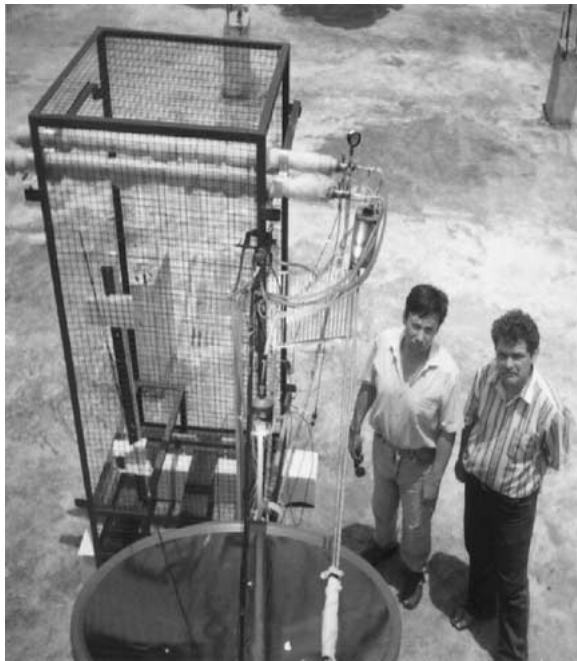
Figure 3. General view of the solar solid sorption refrigerator.
